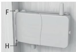
2. Next to the adhesive spacer (H), position the trim (F) on the door frame. The spacer marks the minimum distance between the lock and the trim. If both these parts are not at the same height, you must use the shims (C) to wedge the lock as shown in step 4.
