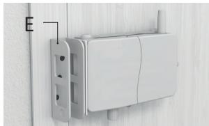
**2.** Next to the adhesive spacer (H), position the bolt storage part (E) on the door frame. The spacer marks the minimum distance between the lock and the bolt storage part. If both these parts are not at the same height, you must use the shims (C) to wedge the lock as shown in step 4.
