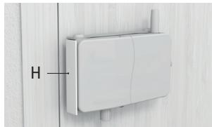
**1.** Calculate the position where you want to install the lock, always inside the door. Place the adhesive spacer (H) as shown in the image, stuck to the body of the lock.
