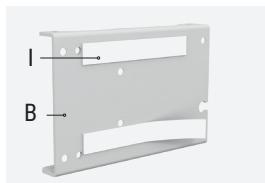
3. Fix the adhesive strips (I) to the rear of the base plate (B) or the shims (C) to suitably position it on the door before drilling.
